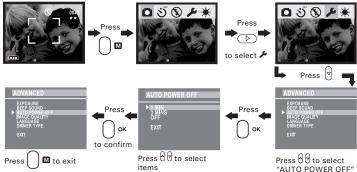
Auto power off is automatically disabled under the following condition: while the camera is connected to a computer or other external devices.
